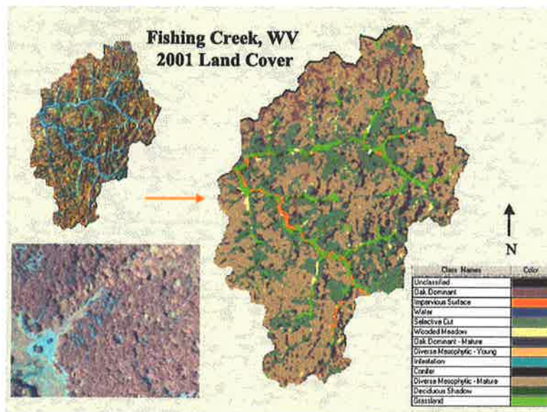
Figure 8. Land-cover classification for Fishing Creek, West Virginia using Landsat data aided by multispectral imagery that revealed wooded meadows in previously logged areas.
