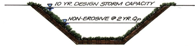
(a) DRAINAGE CHANNEL
