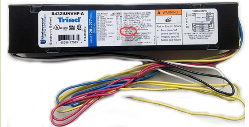
A typical Non-PCB containing fluorescent light ballast. The ballast has a "No PCBs" marking on the top of the ballast and the text "electronic ballast". Only magnetic fluorescent light ballasts contained PCBs.
